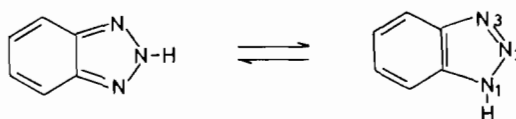
Fig. 1. Structures of two tautomers of benzotriazole (BTAH), 1. The deprotonated species is abbreviated as BTA.
